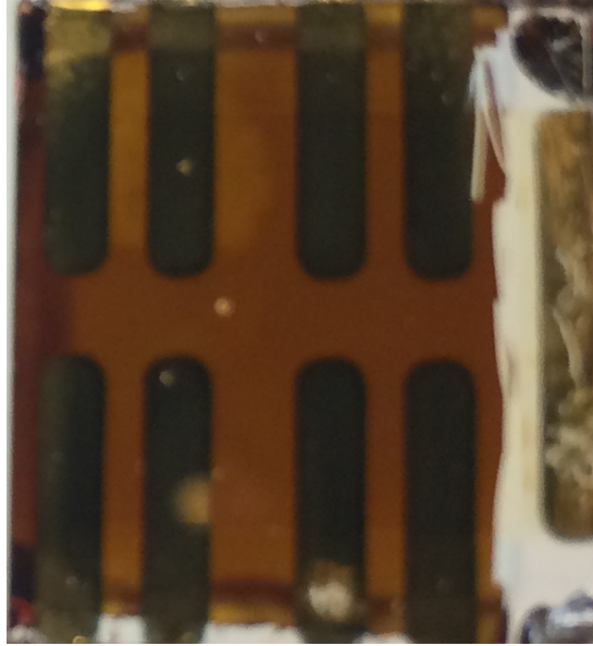
FIGURE 32. A photograph of degraded \text{CH}_3\text{NH}_3\text{Pb}(\text{I}_{0.6}\text{Br}_{0.4})_3 solar cells. Note the paler patch in the upper left hand corner of the cell. The two cells in this region were not used because this \text{PbI}_2 rich section shunted the cells. This region seemingly contributes to the high baseline of \text{PbI}_2 seen from t=0 in this cell. Subsequent evolution apparent in XRD was not visually recorded anywhere, but there is no guarantee that it took place within the cells used for electrical characterization as the region of sensitivity for XRD would have included almost all the devices.
