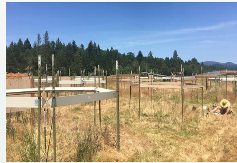
Heat & Precipitation: heating by 2.5° C with added irrigation to match soil moisture of control plot
