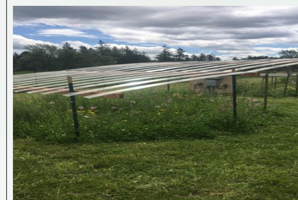
Drought: Acrylic shingles cover plot area and reduce precipitation by 40%
