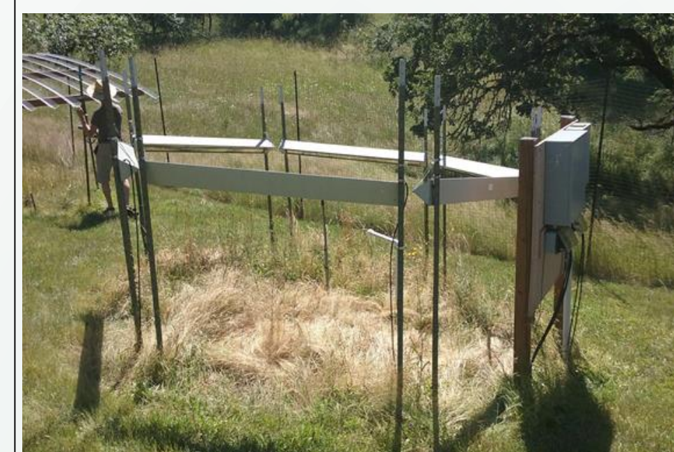
Heat: increase ambient temperature by 2.5° C using 6 infrared heaters
