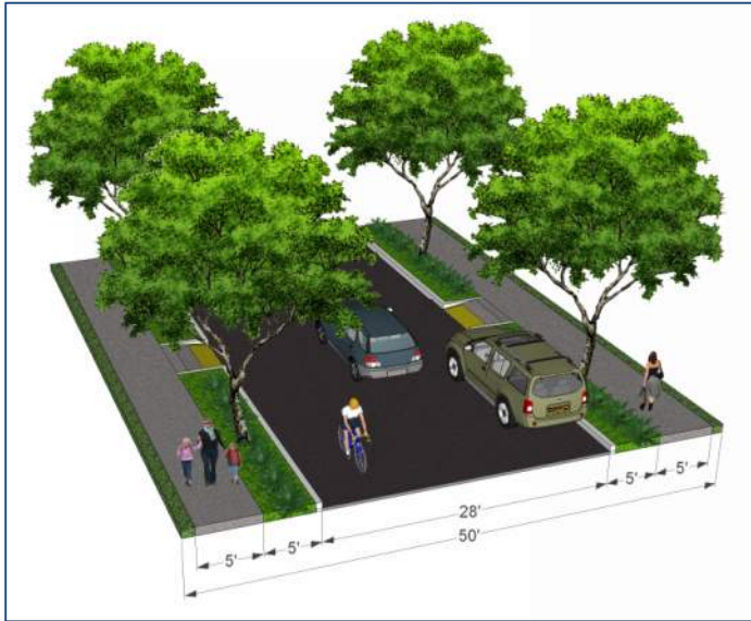
Figure 6: Local Street II - Two Travel Lanes with On-Street Parking on Both Sides
