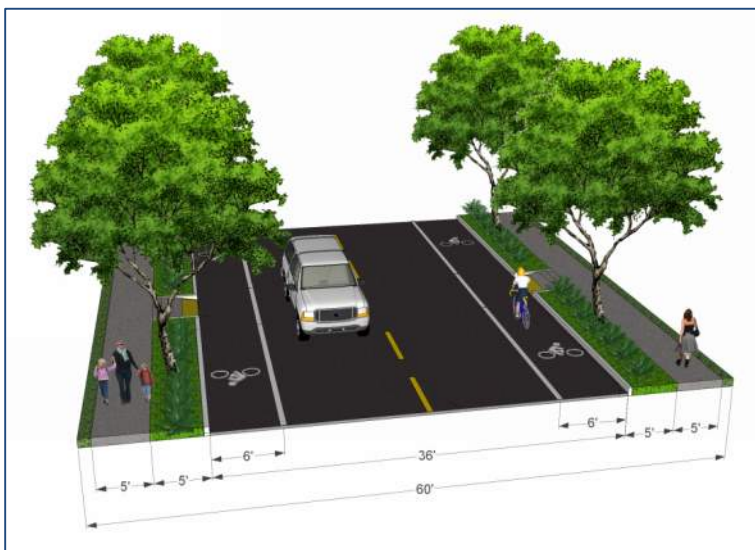
Figure 4: Parkway Collector with Bike Lanes
