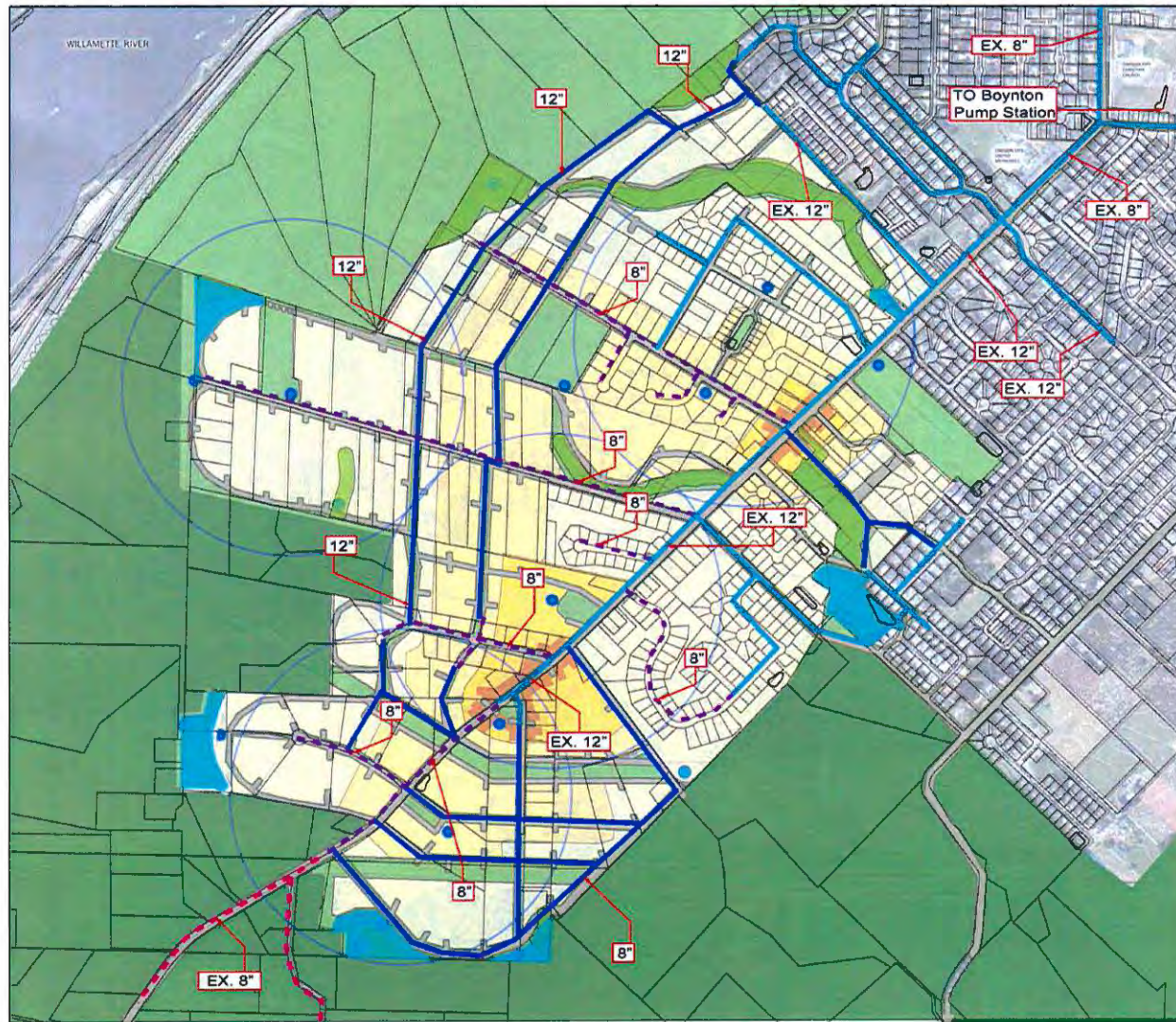
Figure 11. Proposed Water System Improvements
