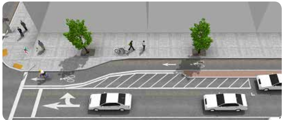
Example of a cycle track bending in towards the roadway and parking restrictions when approaching an intersection
