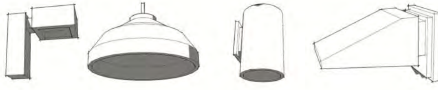
9 Figure 12.50.240-B: 10 Examples of Shielded Light Fixtures
