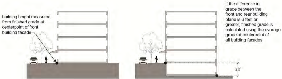
Figure 12.50.140-B: Measuring Building Height on Slopes
