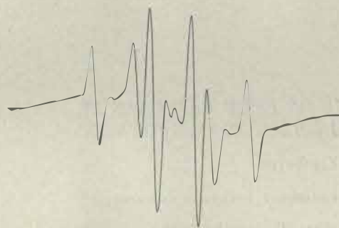
FIG. 1.—The room-temperature ESR spectrum recorded with the magnetic field in the xy plane of an ethyl heptanoate-PHTP crystal. The sharp six-line spectrum is due to the \text{CH}_3(\text{CH}_2)_6\dot{\text{C}}\text{HCO}_2\text{CH}_2\text{CH}_3 radical. The very broad single line in the background is evidently associated with X-ray-damaged PHTP.
