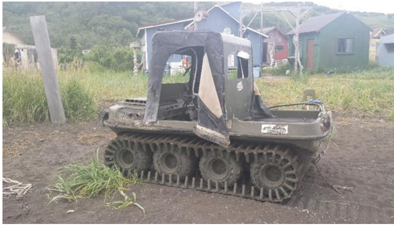
Fig. 9: The Argo, a vehicle used to ride across the mudflats during low tide. Nushagak, Bristol Bay, AK in 2015.
