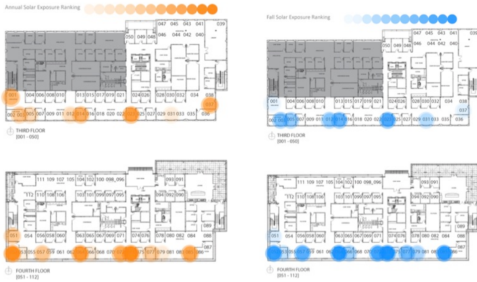
Figure 131: Floor plans showing sampled offices and solar exposure value rankings for annual solar exposure (left) and fall solar exposure (right).
