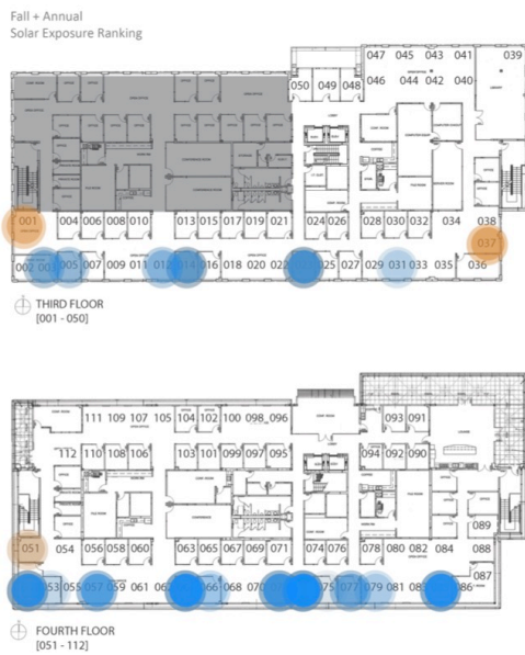
Figure 132: Combined solar exposure value rankings for sampled offices showing fall ranking results (blue) overlaid on top of annual ranking results (orange).
