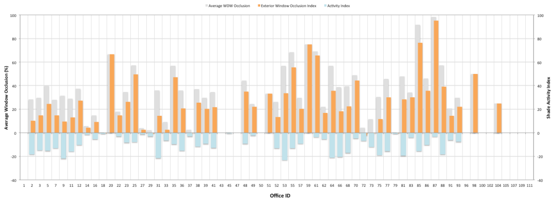
Figure 41: Final exterior window occlusion index plotted for each office in the study population.
