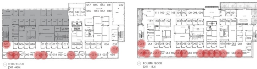
Figure 129: Floor plans showing offices in which solar exposure measurements are taken on the third floor (left) and fourth floor (right).
