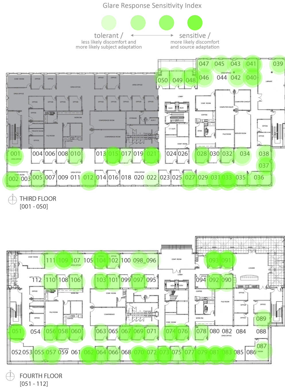
Figure 56: Glare Response Sensitivity (GRS) index results mapped onto floor plans to show spatial distribution of GRS index results.
