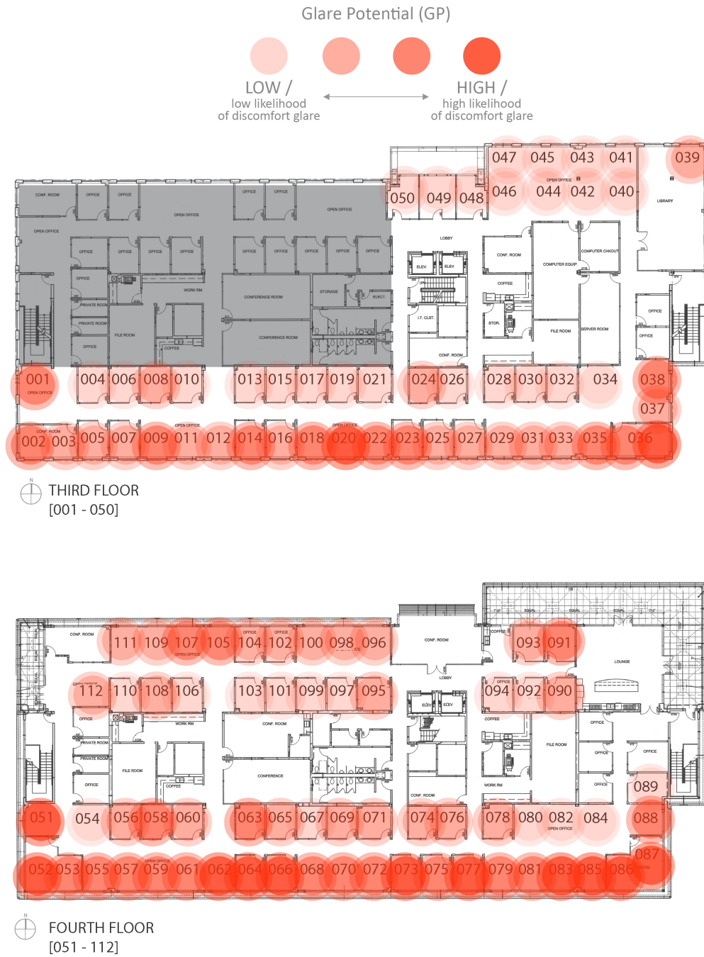
Figure 37: Glare Potential (GP) results shown mapped onto third and fourth floor plans. Saturated icons represent offices with higher GP values.
