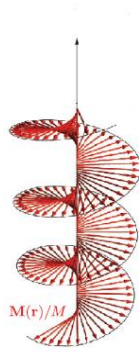
Figure 1.1. Schematic depiction of a global magnetic helix, where there is ferromagnetic order in planes perpendicular to the pitch vector direction. After Ref. [8].
