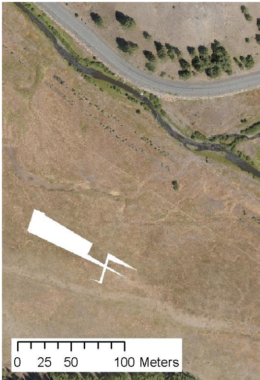
Figure 28: Examples of the effects of missing photo coverage (left) and orthorectification artifacts (right).
