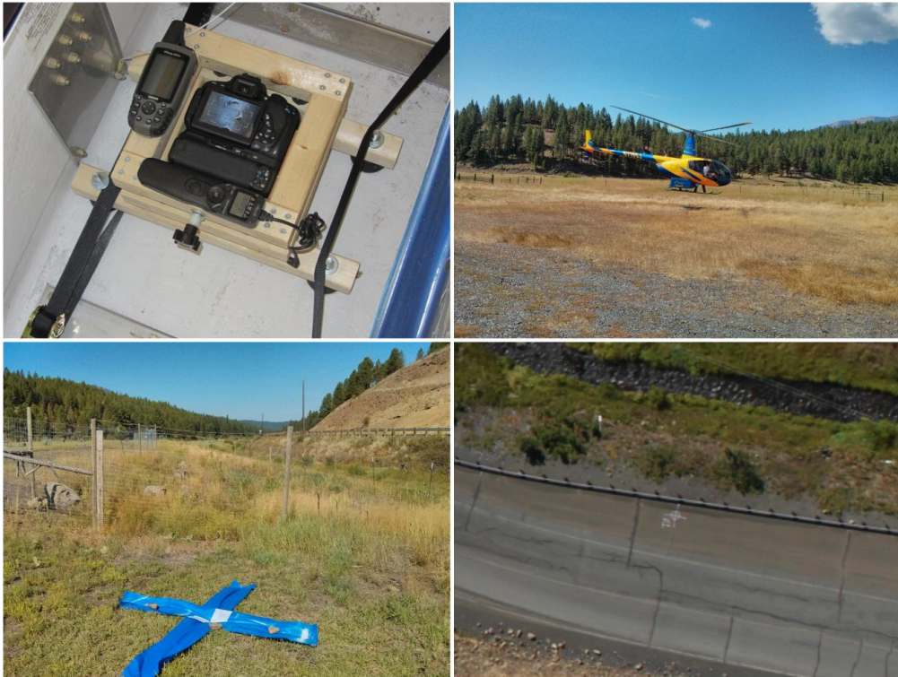
Figure 25: Helicopter aerial photography setup. Canon T5i in the vibration-isolating mount with GPS and intervalometer (upper left). Robinson R44 helicopter at takeoff (upper right). Examples of ground control targets, 1-meter tarps (lower left) and roadside painted targets (lower right).
