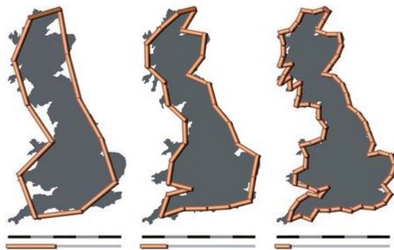
FIGURE 3.4. Evaluating the length of the coastline of Britain at different levels of precision. When the length of the “ruler” used to measure the profile is reduced, the number of rulers needed to encompass the profile increases at a greater rate, yielding a greater number for the measured total length. Image licensed under Creative Commons CC BY-SA 3.0 ( creativecommons.org/licenses/by-sa/3.0/us ) by Wikipedia contributor Avsa.
