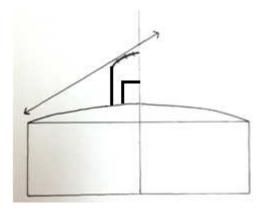
Figure 29: Cross section of a viol at the bridge, displaying projected bow clearance against the instrument's body according to bridge curvature and height.
