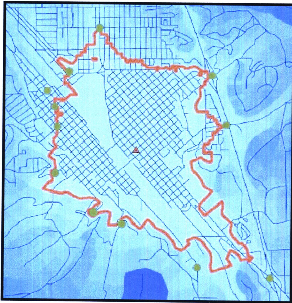
Figure 6. This map shows how the calculated response time (line) for Fire Station 1 in Pocatello compares to the tested time (points).
