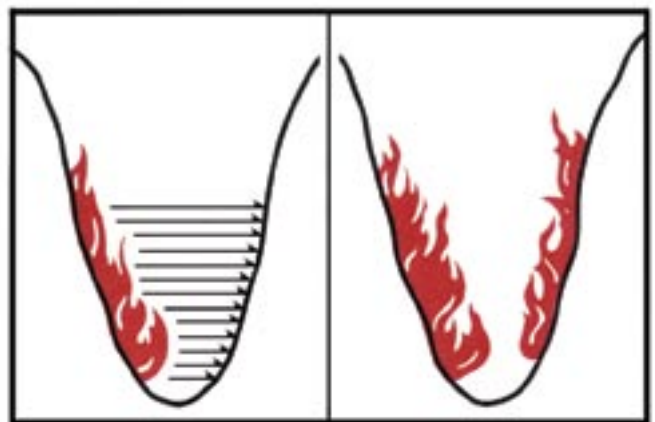
Flashover in V-shaped valley.
