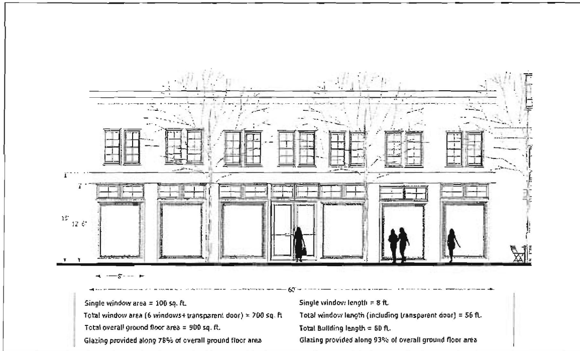
Figure 10A-33-07a. Example of Measuring Window Glazing
