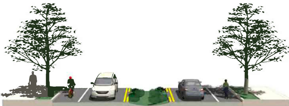
Figure 3-E. Collector 3-Lane Cross Section
