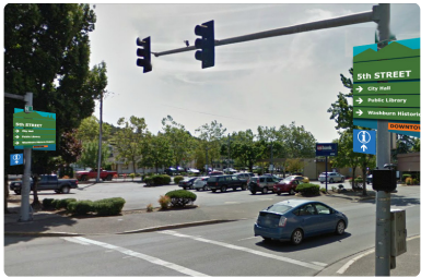
Sign pieces individually mounted on tall poles. Sign design stays consistent throughout city to avoid distraction of drivers. Zone designation is shown with a smaller sign mounted below the directional signage. When placed in one of Springfield’s districts, text indicates location. When not within district boundaries, instead, simple zone name is used.
