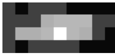
FIGURE 26. Image of a single-mode optical fiber approximately 1.5 mm away from the center of the aspheric imaging system.
