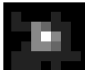
FIGURE 22. Image of a single-mode optical fiber 0.5 mm away from the center of the aspheric imaging system.
