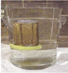
Add modeling clay to the Diet Coke to make it neutrally buoyant
