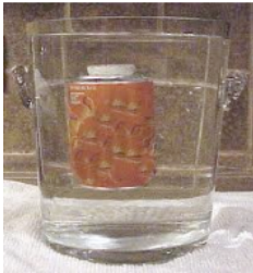
Add styrofoam to the Classic Coke to make it neutrally buoyant
