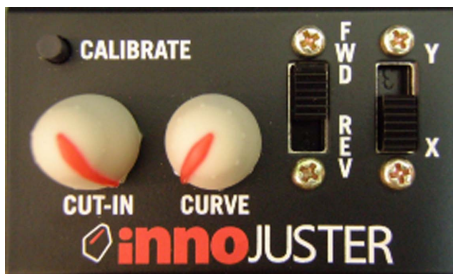
Figure 54: Because the innoFADER has so many adjustments that can be made on it that require taking out the crossfader, the innoJUSTER is a unit that allows users to make those adjustments externally. Image courtesy of Audio Innovate.
