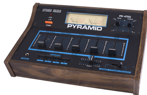
Figure 36: Picture of a Pyramid PR-4700, a mixer with a stiff crossfader that was many DJs' first mixer in the 1980s. Photo by Zane Ritt. Courtesy of the DJpedia Archive.
