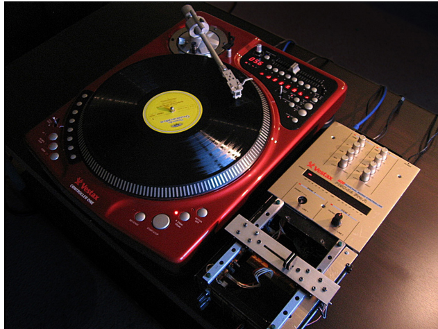
Figure 39: Fretless Fader fitted into a Vestax 06Pro next to a Controller One turntable. Image courtesy of JohnBeez.
