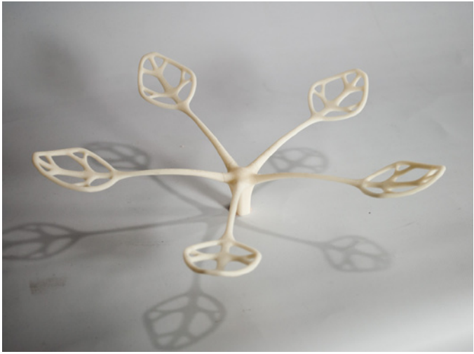
Figures 47 and 48: A small model of the MELAS with all five luminaires. The MELAS light is lit with multiple small LEDs instead of a single light source
