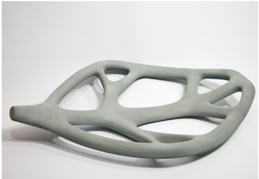
Figures 45 and 46: A model of the MELAS was milled out of foam on a CNC router
