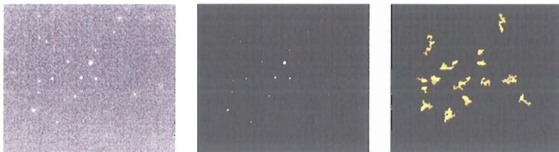
Figure 2.15: Data analysis flow of our video particle tracking procedure. ( Left ) raw fluorescence image of 200nm spheres bound to a freestanding lipid bilayer. The bright spots are the particles. ( Middle ) image with an intensity bandpass filter applied. All pixels with an intensity less than a user chosen threshold are set to zero. At this point the local intensity maxima are cataloged by a simple nearest neighbor comparison. ( Right ) filtered image with Brownian motion tracks overlaid. The track positions are determined by fitting a 2D Gaussian to the local intensity profile in the neighborhood of the local maxima found in the previous step. These trajectories provided position as a function of time for all particles in each sample.
