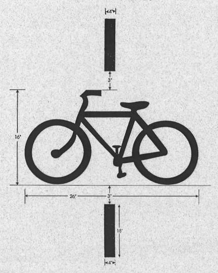
Placing the Bicycle Symbol Stencil in the Most Sensitive Area Over Signal Loops Allows Bicyclists to Trigger Signals in the Travel Lane or Bike Lane
