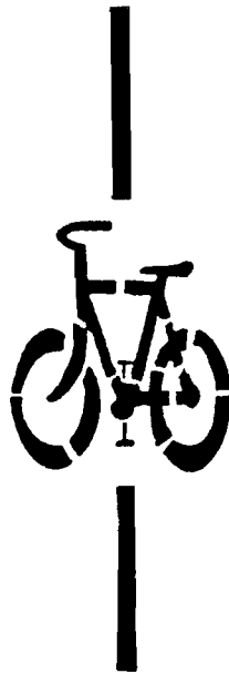
FIGURE 17 - TYPICAL LOOP MARKING
