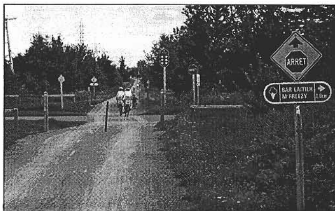
Trail intersections with rural roads require signage on the trail and on the road and traffic control devices to limit access to the trail by motor vehicles.
