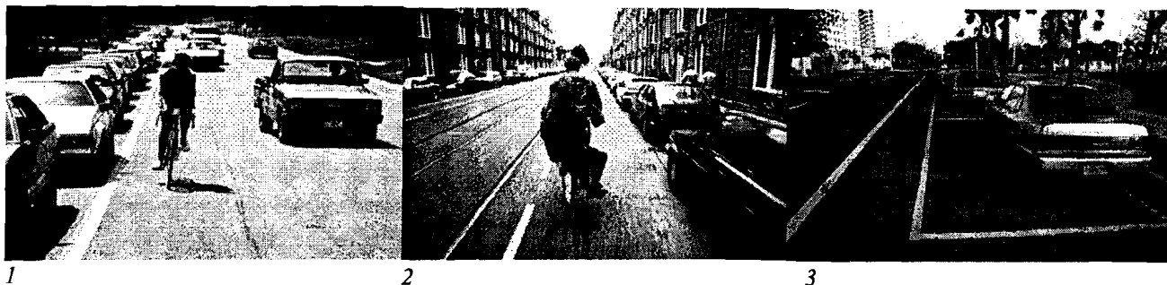
Left to Right: (1) When bicycle lanes are not provided, some motorists and bicyclists make erratic moves. (2) Dutch multi-modal street has near perfect form. Sidewalks, are buffered by orderly parking. Space is delineated for bicycling, tram lines, and bi-directional motorized traffic. (3) Sarasota preserves pleasant bicycling space in new downtown section, (4) Eugene's one-way street has marked bike lane fully separated from parking. Left: Santa Monica's principal roadway provides on-street parking and a full width bike lane.
